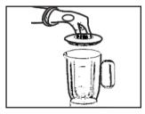
Put the ingredients inside the liquidizer jar or dry grinding Jar and shut the lid by pressing downwards. Also fix the food processor bowl & cover as the machine will not work till the Bowl cover is in place.
