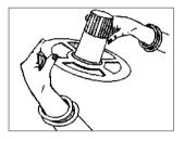
To lock the holder turn anticlockwise
