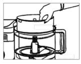
Push down with a juicer pusher. The juice will collect in the bowl where-as the pulp accumulates in the juicer body along with walls of the filter. For best results prepare small quantities at a time and clean the filter frequently. For cleaning, unlock and remove the filter, shake in a bin and wash it under tap water.
