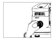
Switch 'ON' the machine. Turn the knob clockwise to the position 1,2 & 3 as per requirement.
