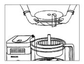
Align the markings provided on the juicer cover and the F.P. bowl, lower the juicer cover on to the bowl and rotate anticlockwise to lock
